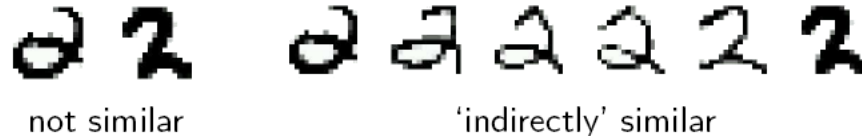
Figure 5.1 Example from NIST handwritten digits recognition. Two handwritten 2's that are dissimilar as measured by Euclidean distance (left). Same handwritten 2's but given a path of other handwritten 2's
